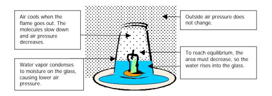
The evaporation of the water to water vapor as the candle burns, and the cooling that occurs when the candle goes out, cause lower air pressure inside the glass than outside. The water is pushed into the glass until equilibrium is reached.)
